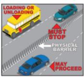
Physical barriers include concrete median barriers, metal median barriers, guide rails, etc.
